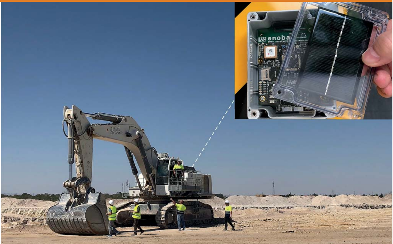
Spin-off project ENOBA integrates intelligent sensors for recording construction vehicle activity data. Photo: ENOBA
