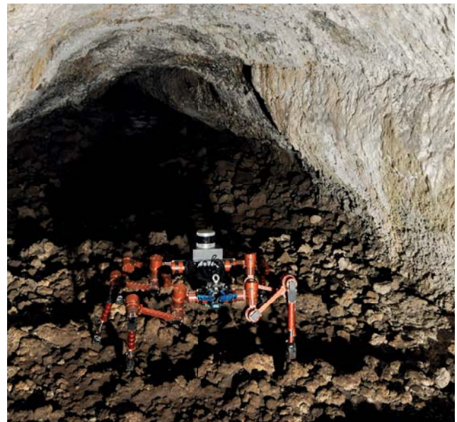
CREX, the six-legged walking robot independently explores a lava cave on Tenerife.
